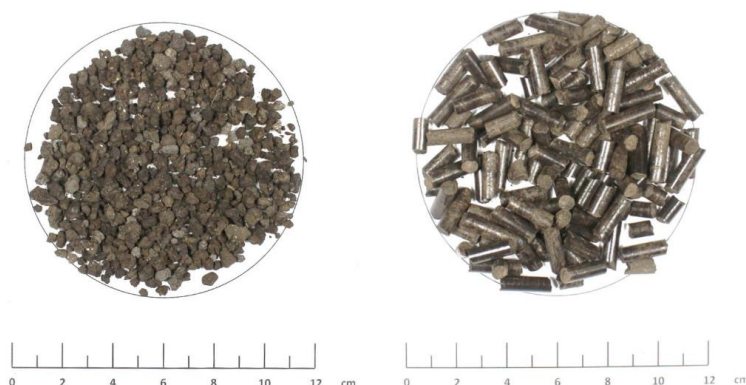
Figure 30 Left: feedstock before pelletising; right: pelletised sludge
