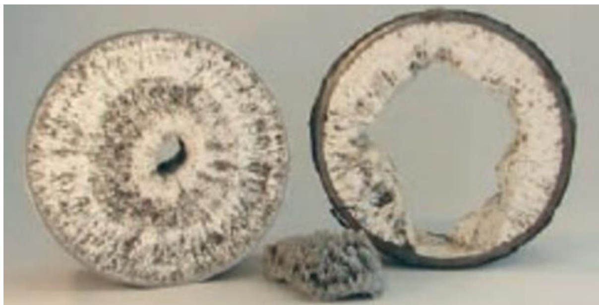
Figure 8: Struvite precipitation in pipes (photo: STOWA)
